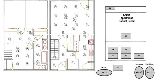
Figure 4: The sensor layout of the Kyoto apartment (left), and the apartment cabinet detail (right)
